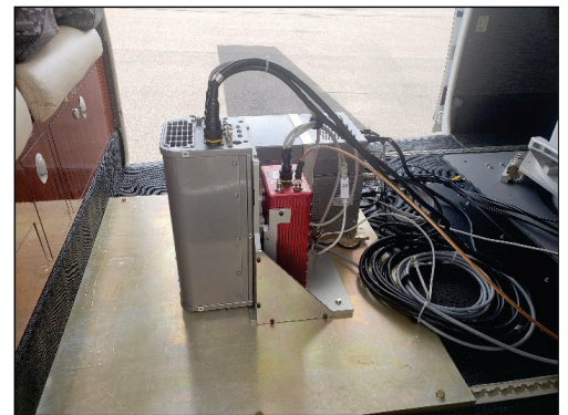
AISA EAGLE II Hyperspectral Sensor Mounted within a Cessna C-208 Caravan
