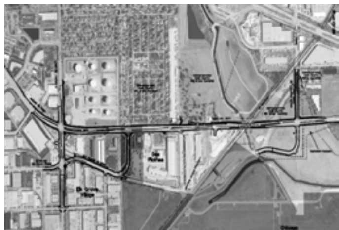
Figure 13. Map of Touhy Avenue improvements. This project reduces congestion and improves reliability through a new grade separation at the Union Pacific Railroad and intersection improvements at Elmhurst Road.
