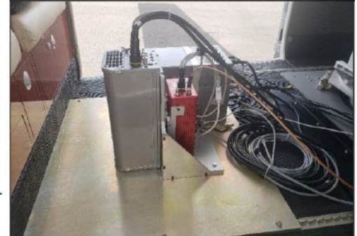
AISA EAGLE II Hyperspectral Sensor Mounted within a Cessna C-208 Caravan
